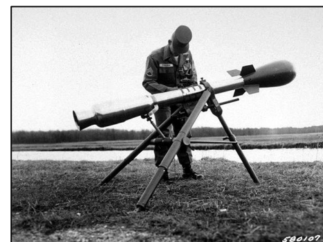
The Davy Crockett Nuclear Bomb, at just 51 pounds, was one of the smallest and lightest nuclear weapons ever deployed by the United States.
